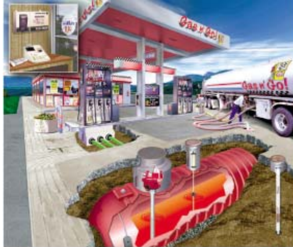
View of tank with STP and ATG probe
