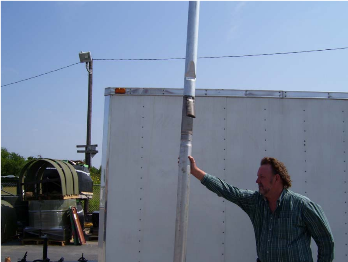
Showing the drop tube with the delivery shut-off valve
