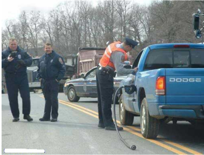
Note nozzle still in gas tank, breakaway on other end
